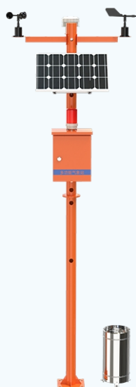
Fixed pole station with solar backup and control box
